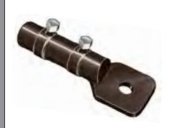
NO. 551-A HEAVY DUTY BRONZE BONDING LUG THAT HAS TWO STAINLESS STEEL SET SCREWS FOR BONDING ALL STANDARD CABLES THROUGH NO. 506 TO FLAT METAL SURFACES. BOLT HOLE SIZE IS NORMALLY 3/8" BUT LARGER HOLES CAN BE FURNISHED WHEN SPECIFIED.
