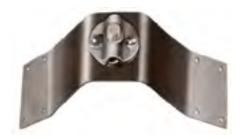
NO. 532-A HEAVY DUTY 31/4" WIDE, COPPER RAISED RIDGE SADDLE. BENDS TO FIT ANY ROOF SLOPE AND HOLDS POINT AND CABLE SLIGHTLY ABOVE THE CENTER OF THE RIDGE. PRESSURE TYPE CABLE CLAMP IS FOR CABLES THROUGH NO. 506. STUD ENGAGES ALL ADAPTER TYPE POINTS. (USE NO. 533 ATTACHMENT TO HOLD AND SUPPORT THE CABLE BETWEEN POINT LOCATIONS.)
