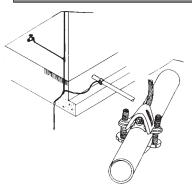
**NO. 240**—A CAST BRONZE PIPE BONDING CLAMP WITH BIMETAL PLATING TO PREVENT CORROSION. THIS CLAMP ACCEPTS CABLES THROUGH NO. 506 AND PIPE OR TUBE DIAMETERS UP TO 1½" O.D. MAXIMUM. USED FOR BONDING MAIN SIZE CONDUCTORS TO MAIN WATER SERVICE, PIPING, OR ELECTRICAL CONDUITS, ETC.
