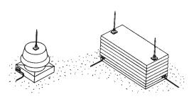
NO. 76MT-A FULLY BIMETAL PLATED 2" WIDE COPPER BASE FOR MOUNTING ALL ADAPTER TYPE AIR TERMINALS ON MECHANICAL EQUIPMENT WHERE CONDUCTOR INTERCONNECTS ARE NOT REQUIRED.
