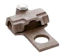
NO. 706RDC—A COMBINATION CABLE SUPPORT AND BONDING CLAMP WITH A 5/8" CLEARANCE HOLE. DEVELOPED FOR USE ON BOLTED STRUCTURES SUCH AS RADOMES, METAL STRUCTURE COVERS, AND CABLE TRAYS, ETC., WHERE STRUCTURAL BOLTS SERVE TO MOUNT THIS FITTING. PRESSURE CAP CONNECTOR ALLOWS FOR CONTINUOUS CABLE ROUTE. FOR CABLES THROUGH NO. 506.
