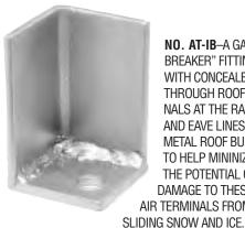
NO. AT-IB—A GALVANIZED STEEL "ICE BREAKER" FITTING USED WITH CONCEALED THROUGH ROOF AIR TERMINALS AT THE RAKE EDGE AND EAVE LINES OF METAL ROOF BUILDINGS TO HELP MININIZE THE POTENTIAL OF DAMAGE TO THESE AIR TERMINALS FROM
