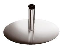
NO. 746M—A PURE COPPER THROUGH ROOF FLASHING THAT HAS AN 8" DIAMETER BASE WITH A  $\frac{7}{8}$ " DIAMETER X 8" TALL COPPER TUBE. COMES WITH EPDM RUBBER SEAL.
