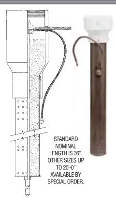
NO. 236E-THE THOMPSON "ENHANCER" REDUCES THE RESISTIVITY OF THE SOIL SURROUNDING THE GROUND ROD. THIS GREATLY INCREASES THE EFFICIENCY OF THE GROUNDING SYSTEM. REDUCTION OF GROUND RESISTIVITY IS ESPECIALLY IMPORTANT IN AREAS OF POOR SOIL CONDUCTIVITY AND/OR SHALLOW DEPTH. UNDER THESE CONDITIONS. OF CROUND SELECTABLES OF UP TO 2007, OR MODE
