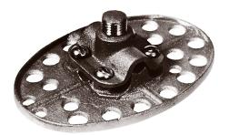
NO. 688C-A HEAVY DUTY CROSS RUN POINT BASE FOR ADHESIVE MOUNTING ON FLAT ROOFS WHERE AIR TERMINALS AND CROSS RUN CABLES ARE JOINED. FITS ALL CABLES THROUGH NO. 506. EXTERNAL STUD ACCEPTS ALL ADAPTER TYPE POINTS.
