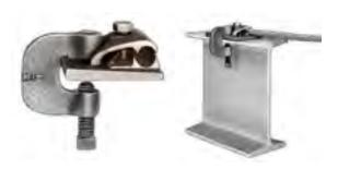
NO. 701X-A HEAVY DUTY FORGED STEEL "C" CLAMP WITH BRONZE BONDING PLATE FOR CABLES THROUGH NO. 506 TO STRUCTURAL STEEL PURLINS, CHANNEL IRON, "I" BEAMS, OR ANGLE IRONS. HAS A PREMIUM DIE CAST BOLT PRESSURE TYPE CABLE CLAMP. FITS STRUCTURAL STEEL UP TO 1" THICKNESS AND HAS 9 SQUARE INCHES OF BONDING SURFACE.
