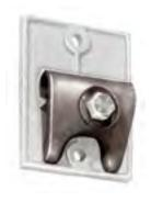
**NO. 702**–A PREMIUM DIE CAST BRONZE BONDING PLATE WITH 8 SQUARE INCH BIMETAL PLATED CONTACT AREA. THE PRESSURE TYPE CABLE CONNECTOR IS FOR CONDUCTORS THROUGH NO. 506. THIS PLATE WILL ACCOMMODATE EITHER A "DEAD-END" OR CONTINUOUS THROUGH CABLE ROUTE. THE TWO HOLES WILL FIT EITHER SHEET METAL SCREWS OR  $\frac{1}{4}$ " MACHINE SCREWS.
