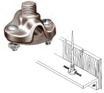
**NO. 636**—A CAST BRONZE BASE FOR MOUNTING ON ANGLES OR CHANNELS AT SCREEN WALLS, ETC. THE MOUNTING BOLTS SECURE THE PRESSURE TYPE CABLE CLAMP THAT ACCEPTS CONDUCTORS THROUGH NO. 506. THE EXTERNAL STUD ACCEPTS ALL ADAPTER TYPE POINTS.
