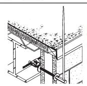
NO. 27DG—A RIGHT ANGLE BASE OF MACHINED BRASS THAT PROVIDES A TRANSITION FROM A HORIZONTAL ½" RISER TO LESS ADAPTER TYPE AIR TERMINALS. (NO. 55LA, ETC.) INCLUDES A SET SCREW TO LOCK THE POINT IN A VERTICAL POSITION. AVAILABLE IN ½" DIAMETER ONLY.
