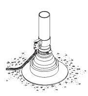
NO. 800-A 1" WIDE BONDING STRAP OF TINNED COPPER WITH A PREMIUM DIE CAST PRESSURE TYPE CABLE CLAMP FOR BONDING TO ROOF VENTS AND PIPING, ETC., UP TO 4" O.D. CABLE CONNECTOR IS FOR SIZES THROUGH NO. 507. (NOT FOR USE AS MAIN WATER SERVICE BOND.) LONGER STRAPS CAN BE FURNISHED FOR LARGER PIPES. (SEE BELOW)
