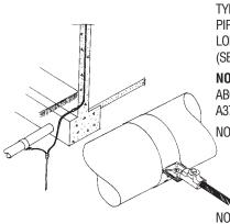
NO. 704-AN ADJUSTABLE 2" WIDE TINNED COPPER BONDING STRAP WITH A PREMIUM DIE CAST PRESSURE TYPE CABLE CONNECTOR FOR CABLES THROUGH 506. FITS PIPE SIZES THROUGH 4" AND O.D. SIZES THROUGH 4½". LONGER STRAPS CAN BE FURNISHED FOR LARGER PIPES. (SEE BELOW.)
