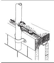
**NO. 802**–A U-BOLT TYPE PIPE BONDING CLAMP WITH CAST BRONZE CABLE CONNECTION AND 5%6" STAINLESS STEEL U-BOLT. CLAMP ACCEPTS ALL CABLES THROUGH NO. 507 AND A MAXIMUM PIPE O.D. OF 1 7%6". ALSO USED TO SUPPORT AIR TERMINALS ON VERTICAL PIPE MASTS OR CONDUIT MOUNTED LIGHTS. ETC.
