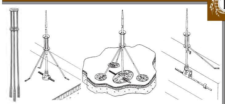
GALVANIZED STEEL TRIPOD BRACES HAVE 1/4" DIAMETER LEGS AND ARE FOR USE WITH 3/8" THROUGH 5/8" DIAMETER AIR TERMINALS. MOUNTING FEET ARE FIELD FORMED AND CAN BE SECURED WITH BOLTS, SCREWS OR NAILS AS REQUIRED.
