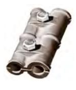
NO. 744-A HEAVY DUTY 3½" LONG BIMETAL PARALLEL CLAMP USED AS A BIMETALLIC CONNECTOR FOR JOINING ALUMINUM AND COPPER CABLES NO. 32 THROUGH NO. 506 TO NO. A24 THROUGH NO. A37 ALUMINUM CABLES.
