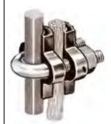
NO. 430B—A U-BOLT PARALLEL CLAMP OF CAST BRONZE USED FOR A PARALLEL CONNECTION FROM EITHER ONE OR TWO CABLES OR RODS THROUGH 5/8" DIAMETER TO ANOTHER CABLE OR ROD. U-BOLT, NUTS, AND WASHERS ARE STAINLESS STEEL.
