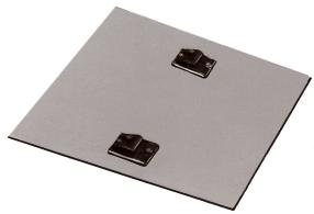
NO. 233M—A SOLID COPPER GROUND PLATE USED WHERE SHALLOW OR ROCKY TOPSOIL CONDITIONS PRECLUDE THE USE OF DRIVEN GROUND RODS. THIS GROUND PLATE IS 18" X 18" X 20 GAUGE THICK AND COMES COMPLETE WITH TWO PREMIUM DIE CAST BOLT PRESSURE TYPE CABLE CONNECTIONS FOR CABLES THROUGH NO. 506.
