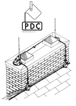
NO. 673-A COMPLETE CHIMNEY POINT ASSEMBLY FOR MOUNTING ON THE TOP OF THE CHIMNEY CAP. INCLUDES A LEAD COATED NO. 611 BASE AND LEAD COATED NO. 55 1/2" X 12" SOLID COPPER POINT WITH BASE ADAPTER. PREMIUM DIE CAST CLAMP ACCEPTS CABLES THROUGH NO. 506.
