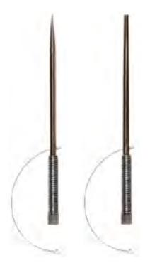
NO. 55SP-FLEXIBLE AIR TERMINALS FOR USE WHERE WINDOW WASHING OR OTHER MOVABLE EQUIPMENT CONFLICTS WITH FIXED AIR TERMINAL. ADAPTER FITS ALL EXTERNAL STUD TYPE BASES. SOLID POINT PORTION IS ½" DIAMETER COPPER WITH NICKEL PLATED TIP. OVERALL HEIGHT IS 12". THE HEAVY STAINLESS STEEL SPRING PROVIDES A 90° TILT IN ANY DIRECTION. COMES COMPLETE WITH A STAINLESS STEEL SAFETY TIE-OFF CABLE WITH LUG FOR ATTACHING TO BOLT AT BASE.
