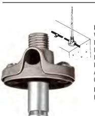
**NO. 78**—A ONE BOLT BRONZE BASE WITH PRESSURE TYPE CABLE CONNECTION FOR INSTALLATION ON FLAT MASONRY. COMPLETE WITH STAINLESS STEEL MACHINE SCREW AND \$\(^{5}\)16" PAK-TITE ANCHOR. STUD ENGAGES ALL ADAPTER TYPE POINTS. ACCEPTS CABLES THROUGH NO. 506.
