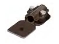
**NO. 645**—A HEAVY DUTY BONDING LUG FOR NO. 507 CABLE WITH 2 SCREW PRESSURE CABLE CLAMP WHICH HAS 2" OF CONTACT LENGTH.
