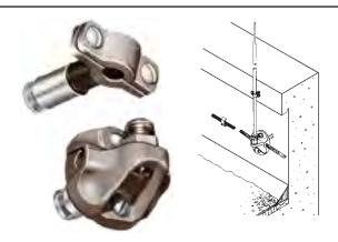
NO. 569-A HEAVY DUTY BRONZE PARAPET WALL BASE WITH EXTERNAL STUD FOR ALL ADAPTER TYPE POINTS. COMES COMPLETE WITH MACHINE SCREWS AND ONE 3/8" PAK-TITE ANCHOR. HOLDS POINTS AT RIGHT ANGLES TO CABLE. USE NO. 574, 575, OR 576 TO SUPPORT UPPER PART OF POINTS. CLAMP ACCEPTS CONDUCTORS THROUGH NO. 506.
