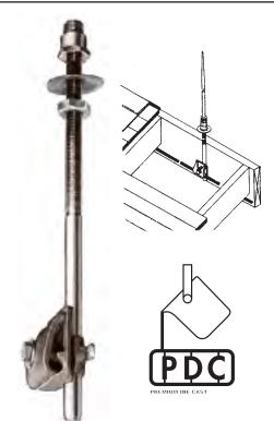
MO. 685-A THROUGH ROOF BASE FOR CONCEALED MOUNTING AT ROOF RIDGE LOCATIONS. ASSEMBLY INCLUDES AN ALL THREAD ½" X 12" LONG RISER BAR, PREMIUM DIE CAST BRONZE CABLE CLAMP FOR CONDUCTORS THROUGH NO. 506, LEAD WASHER FOR WEATHER SEAL ABOVE THE ROOF, HEX NUT, AND FLAT WASHER TO SECURE RISER BELOW THE ROOF, AND NO. 28M ADAPTER FOR ALL ADAPTER TYPE AIR TERMINALS.
