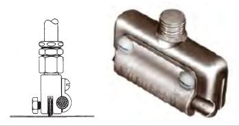
**NO. 691**—A CLAMP TYPE POINT BASE FOR FASTENING TO STANDING SEAM METAL ROOFS WITHOUT THE USE OF MECHANICAL FASTENERS. BOLT PRESSURE CLAMP ACCEPTS CABLES THROUGH NO. 506. EXTERNAL STUD ACCEPTS ALL ADAPTER TYPE AIR TERMINALS.
