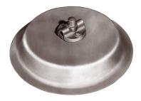
NO. 694-THIS PAN TYPE POINT BASE IS FOR FLAT ROOFS. INCLUDES A COMBINATION POINT TO CABLE BASE CONNECTOR WITH EXTERNAL STUD FOR ALL ADAPTER TYPE POINTS. ACCEPTS CABLES THROUGH NO. 506. THE PAN IS FILLED WITH CEMENT ON THE JOB AND IS INVERTED AFTER THE CEMENT SETS. NO. 589 PAN-TYPE CABLE SUPPORTS ARE USED IN CONJUNCTION WITH THIS BASE. CAN BE USED WITH OR WITHOUT ADHESIVE. OVERALL WEIGHT HOLDS BASE AND CABLE SUPPORTS IN PLACE.
