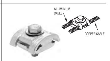
**NO. 141T**–A SPECIALLY PLATED PARALLEL SPLICER USED AS A BIMETAL CONNECTION BETWEEN COPPER AND ALUMINUM CONDUCTORS FROM NO. 29X/NO. A24 THROUGH NO. 507/NO. A507.
