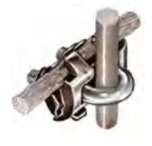
NO. 493-THIS 5/16" STAINLESS STEEL U-BOLT TYPE ROD TO CABLE CLAMP IS A VERY VERSATILE CONNECTOR FOR CLAMPING ALL MAIN SIZE CABLES FROM NO. 29X THROUGH NO. 507 TO GROUND RODS THROUGH 3/4" DIAMETER. THIS CLAMP CAN ALSO BE USED TO CONNECT AIR TERMINALS, RISER BARS, REINFORCING RODS, AND SMALL PIPING (THROUGH 7/8" DIAMETER) TO CABLES.
